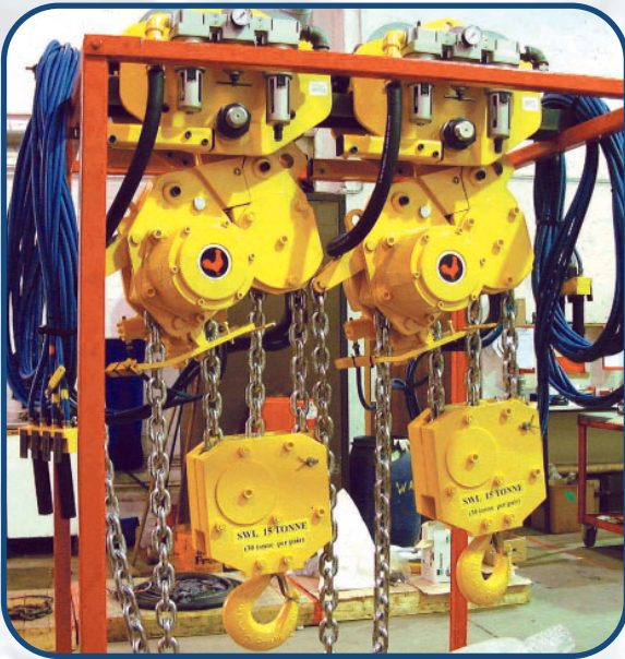
BOP handling system
